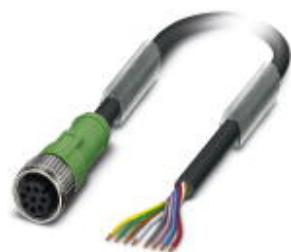
Sensor/actuator cable, 8-position, PUR halogen-free, black-gray RAL 7021, shielded, free cable end, on Socket straight M12, A-coded, cable length: 5 m, Shield not connected to knurl
